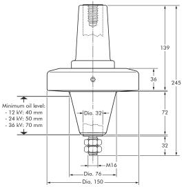
6/10 (12) kV 6.35/11 (12) kV 8.7/15 (17.5) kV 12/20 (24) kV 12.7/22 (24) kV 18/30 (36) kV
