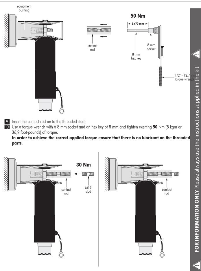
III Install the M16 threaded stud into the bushing interface.
