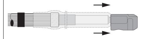
After tightening the contact, slide the cable reducer up until it butts against the contact.
