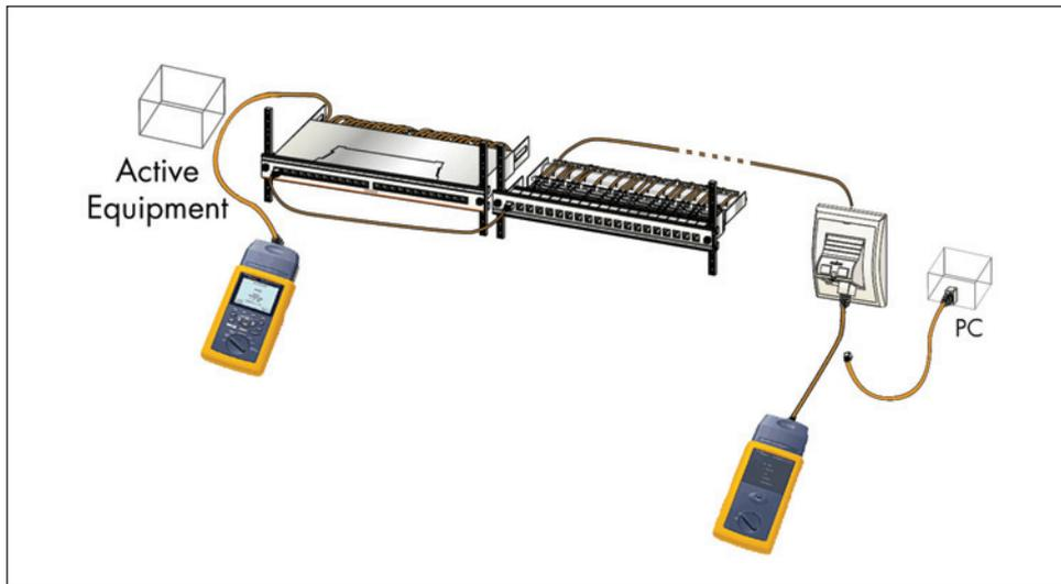
Figure 2.2: Testing at 3 connector Cross connect - TO model
