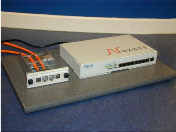
Nexans set up a GG45-Cat7 network of two Category 7 links for each eight persons. The installation time constraint of 5 hours, in a hotel environment, was successfully respected.
